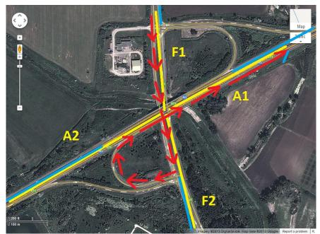
In this example, the vehicle turns left, leaving the main road (Section F1) and driving onto the motorway (Section A1) but, because the unit tolled sections (F1, F2, A1, A2) start from the mathematical centre of the intersection, the Section Matching of the unit tolled sections (F2) and (A2) does not have to be performed for the loop used for turning to the left.
